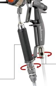
For quick cleaning when the nozzle is blocked: simply insert the nozzle the other way round and flush
